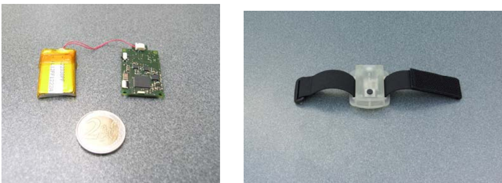
Figure 3: Top views of the wrist hand sensor unit (PDInerUnit). The left view shows the internal parts of the unit, namely: battery and PCB (printed circuit board). The right view shows the integrated unit which is supposed to be worn around the hand wrist.
