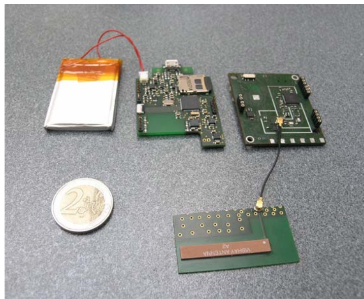
Figure 5: Top view of the PDInerRFIDUnit. It shows two PCB board, left part is inertial sensor unit and the right part is RFID reader with antenna.
